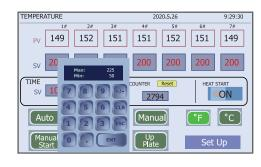
Note: Setting the press temperature to above 400°F (200°C) may cause a fire hazard.
